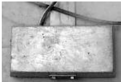
Zinc anode with bracket and bonding wire
